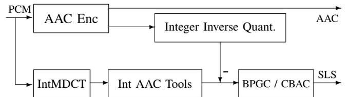
Fig. 2. Basic building blocks of combined AAC/SLS encoder
