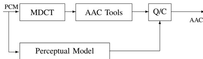
Fig. 1. Basic building blocks of AAC encoder
