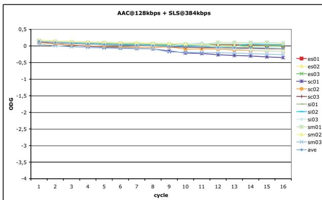
Fig. 5. Test results: AAC + SLS in tandem coding
