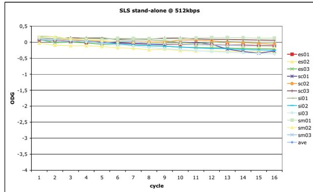
Fig. 6. Test results: SLS stand-alone in tandem coding
